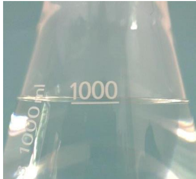
Photo 2: Correct 1 liter beaker filling for ECOWASH density measurement.
